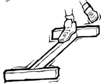
Place the two-by-fours on their thinner edges, forming an H (see illustration). Center and nail the shorter boards onto the ends of the longest two-by-four. Sand down the entire surface, making sure there are no rough edges or splinters.
